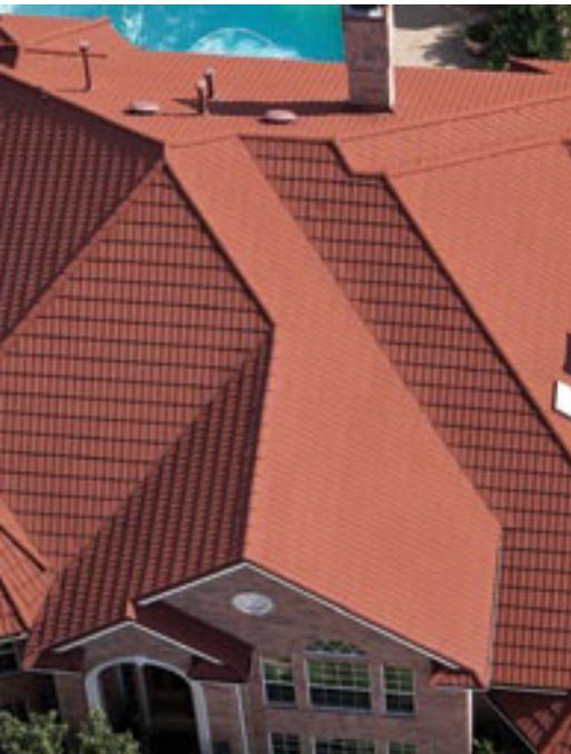
Every SteelROCK panel is formed from 26-gauge Galvalume® steel and covered with natural stone granules that are embedded in a 100% acrylic resin basecoat. The panels are then finished with a clear acrylic over-glaze to seal and protect the stone granules.
