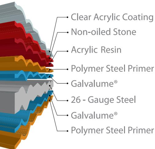
Every SteelROCK panel is formed from 26-gauge Galvalume® steel and covered with natural stone granules that are embedded in a 100% acrylic resin basecoat. The panels are then finished with a clear acrylic over-glaze to seal and protect the stone granules.
